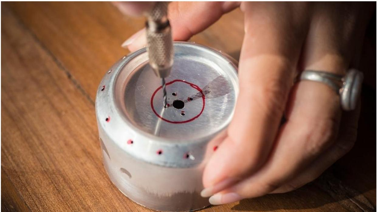
Place a penny in the center of the can bottom and outline it with the marker. Remove the penny and mark a dot in the center of the circle. Mark four additional holes around the center dot. Drill the center with a 3/16" bit and the four outside holes with a 1/16" bit.
