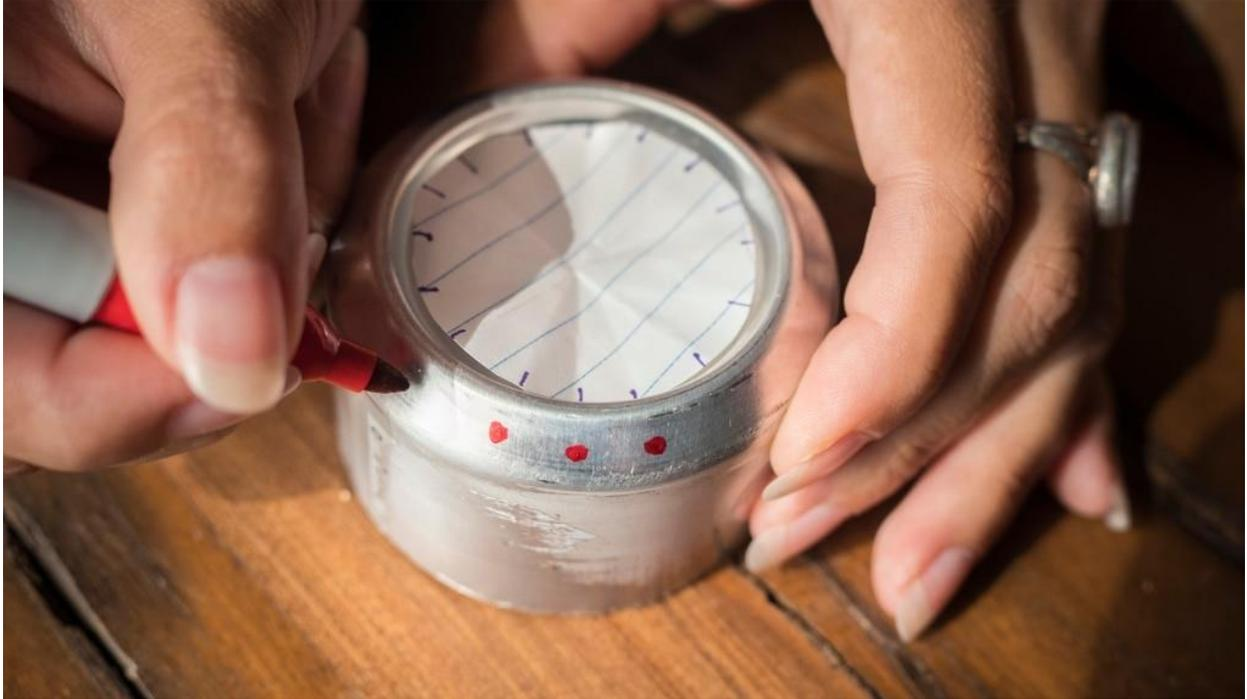
Turn one can upside down, and place a piece of paper on it. Trace a circle on the paper using the bottom of the can as a guide. Cut out the circle and fold it in half four times. Unfold and place on the bottom of the can. Use a marker to dot the can at each fold; there should be 16 evenly spaced marks. Drill each dot using a 1/16" drill bit.
